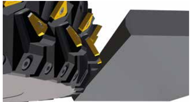
I + V-輪廓 = 附 2 個系列銑刀的X-輪廓 I + V-profile = X-profile with 2 serial cutters
