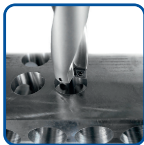
Vollbohren Solid drilling
