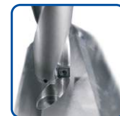
Beveling/drilling at an angle, cutting interruption
