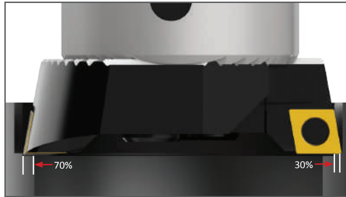
Material removal up to 0.276" - 0.394" (7.00 mm - 10.00 mm) on diameter: 70% roughing 30% finishing
