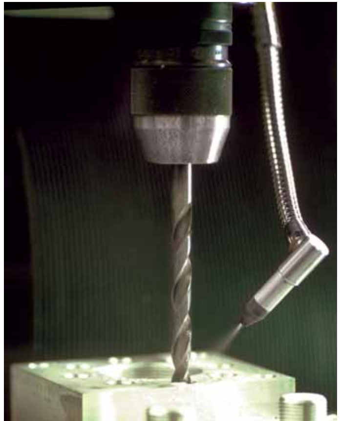
Tool cooling and lubrication in an air cushion
